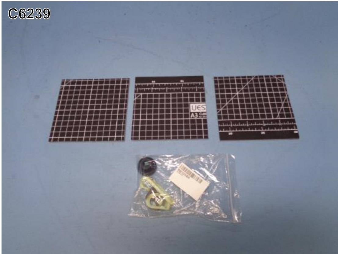
System Equipment – World Anchor Test cards, Calibration Cap and Lens and Lens Clips
